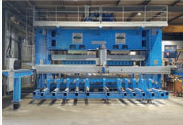
Special double cylinder hydraulic presses for forming of corrugated sheets complete with:
