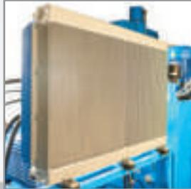
Air hydraulic fluid cooling system
