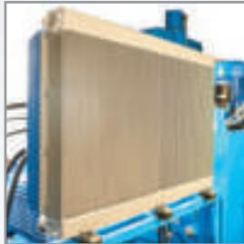
Air hydraulic fluid cooling system
