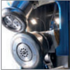
Forming and flanging rolls in alloy steel with surface induction hardening
