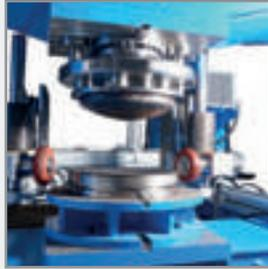
Manipulator wheels with vulcanized coating and hydraulic motorization
