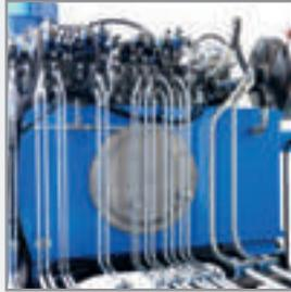
Separate hydraulic power unit with rigid piping
