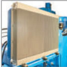
Air hydraulic fluid cooling system
