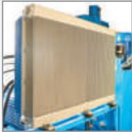
Air hydraulic fluid cooling system
